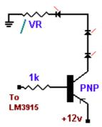
Here there is nothing to write, the LM3915 is ready for this kind of application so you don't need other things...You must only set the variable resistor for a right visualization of volume level.
